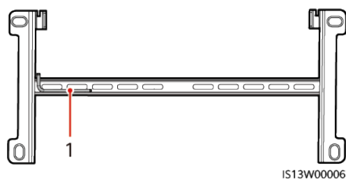
Figure 4-11 Position for binding the security Torx wrench
